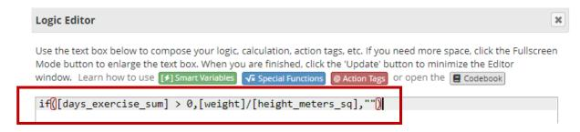
The conditional logic within the 'If' function mimics the branching logic and resolves the resulting error.
